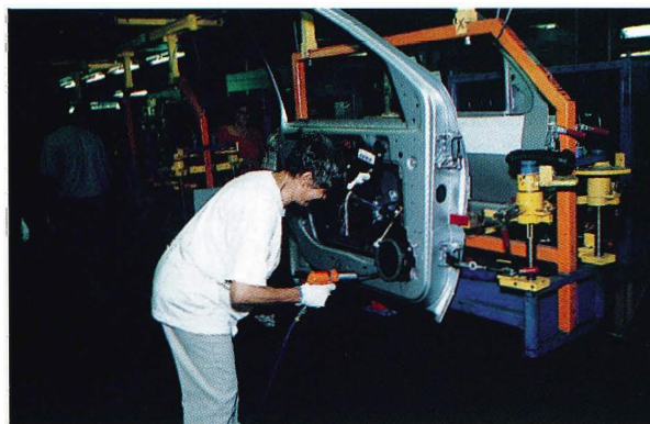
Door plug assembly at GM's Doraville plant.
